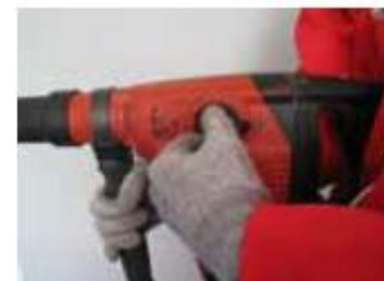
Position perforation percussion
